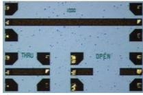
▲ Fig. 4 TRL calibration structures.
