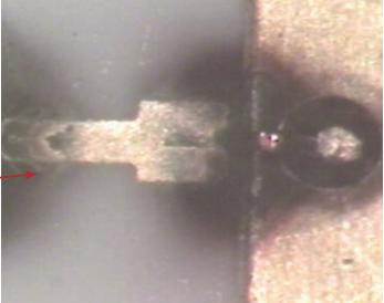
A Photos (normal left, magnified right) show damage to the microwave junction.
