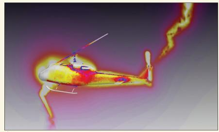
▲ Fig. 3 New capabilities in the HFSS Transient solver make it easy to simulate time domain scenarios, such as ESD and lightning strikes on aircraft.
