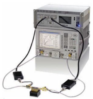
▲ Fig. 1 BILT/IVCAD pulsed IV/S-parameter characterization system.
