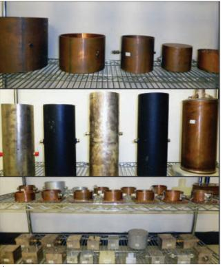
Fig. 7 Custom resonator test cavities.
