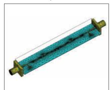
Fig. 7 Composite model of the filter in the WR22 waveguide, including the coax connectors.
